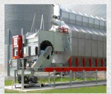
Airlock Package includes a rotary airlock and a TEFC motor and drive mounted and assembled on a heavyduty, galvanized steel airlock base. The drive features a high efficiency in-line gearbox to deliver more torque to the airlock.
