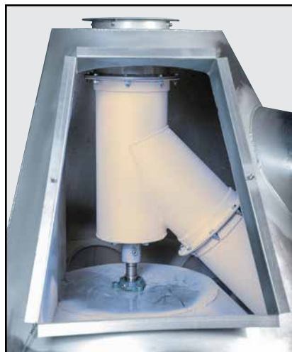
Distributor inner turn spout seen through large access door (with door removed).
