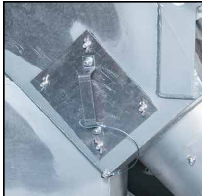
Clean out doors provide easy clean out access as well as rust prevention maintenance.
