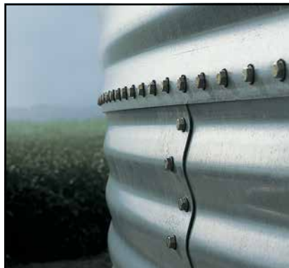
Sidewall Corrugation Options include wide (4 in./102 mm) or narrow (2.66 in./ 68mm) corrugation.
