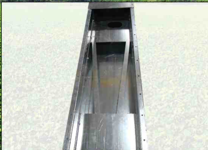
View of grain drop through opening (with covers removed).
