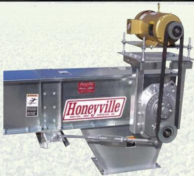
Head and tail sections G-90 galvanized steel, all sprockets with taper lock bushings. Class II Dodge torque-arm type gear reducer installed with over-head motor mount and fixed pitch v-belt drives.
