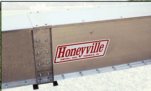
Conveyor trough sections are all G-90 formed galvanized steel with no welding on any exterior panels. Bolted formed channel type trough connections.
