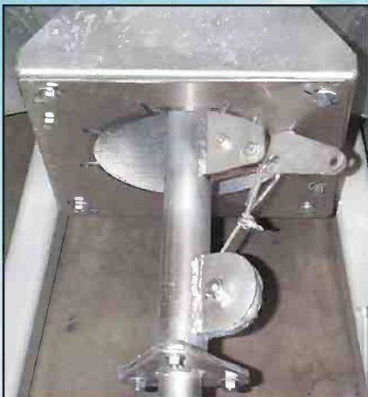
Positive locking index plate located under the distributor for protection from dust and weather.
