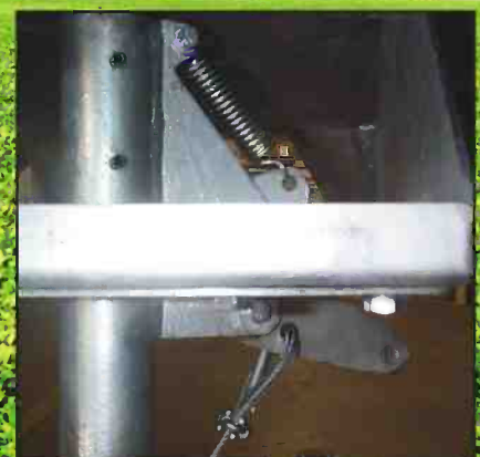
Spring tensioned latch mechanism.
