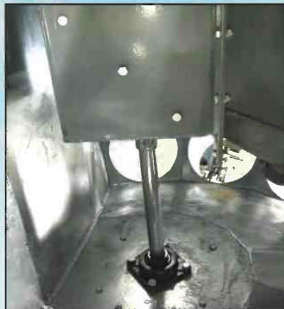
Swing spout rotates on a solid shaft with a flanged block bearing.
